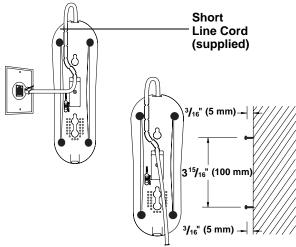
**Note:** The USOC number of the jack to be installed is RJ11C (RJ11W for a wall jack).
